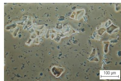
Conglomerates of large precipitates with crystalline and solid structure of vaccine affected by freezing ( $-10^{\circ}\text{C}$ , solidly frozen)
