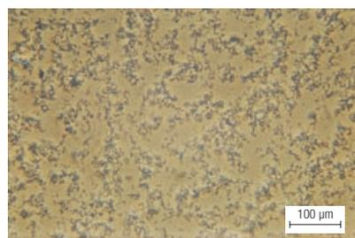
Fine-grain structure of vaccine exposed to  $-10^{\circ}\text{C}$  until slushy (not fully frozen)
