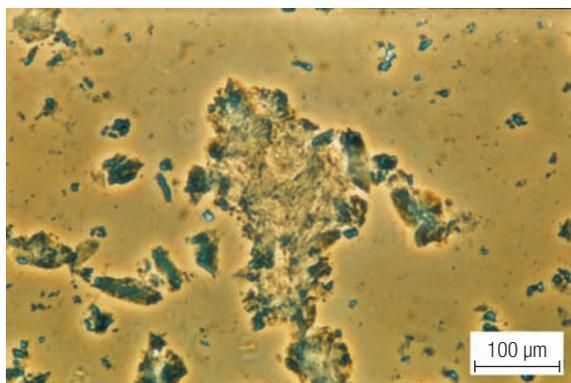
Conglomerates of large precipitates with crystalline structure of dT vaccine affected by freezing (–25 °C) (code 4250942)
