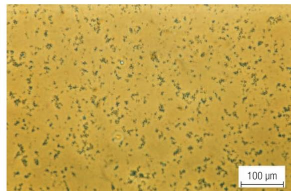
Fine-grain structure of DTP–HepB vaccine exposed to –2 °C for 24 hours (code 1870463)
