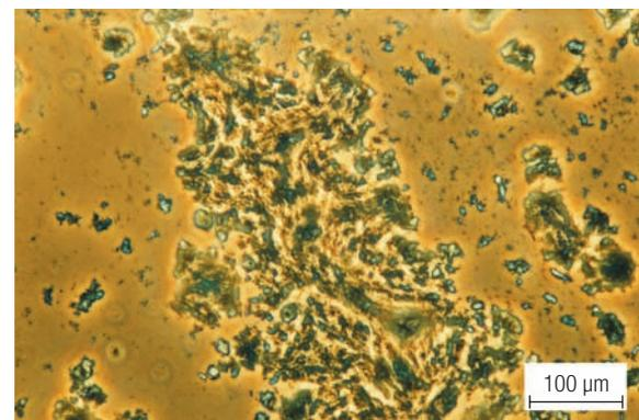
Conglomerates of large precipitates with crystalline structure of DTP–HepB vaccine affected by freezing (–25 °C) (code 1800462)
