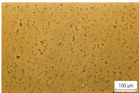
Fine-grain structure of dT vaccine exposed to –2 °C for 24 hours (code 4280943)
