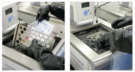
VVMs in sealed pouches transferred to water baths in metal cages to sink
