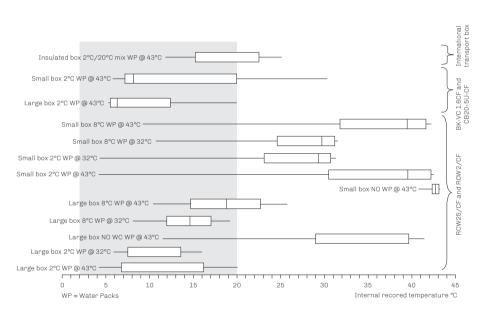
Box and whisker plot of recorded temperatures at all laboratory tests
