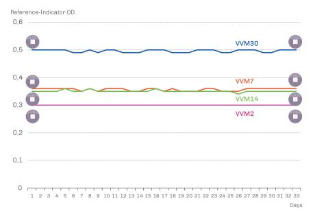
Reference-Indicator OD measurements for VVM2, VVM7, VVM14, VVM30 kept at REFRIGERATOR from 27 January to 28 February 2014 (average temperature +7°C)
