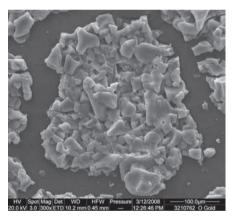
Freeze-damaged DTP-HepB vaccine under SEM 300X with clutters of sediments
