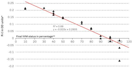
\* Difference between the reflection densitometer reading of the reference ring (R) and active indicator surface (I) in optical density (OD) units
