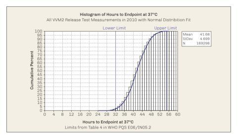
Coefficient of variation (also known as unitized risk) is a normalized measure of "dispersion" of a probability distribution and is used widely in probability theory and statistics. Coefficient variation (CV) of VVM2 reaction at 37°C from the first graph is calculated to be 0.75. Any CV that is <1.0 is statistically considered low-variance.
