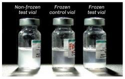
Differentiating the vaccine damaged by freezing through shake test
