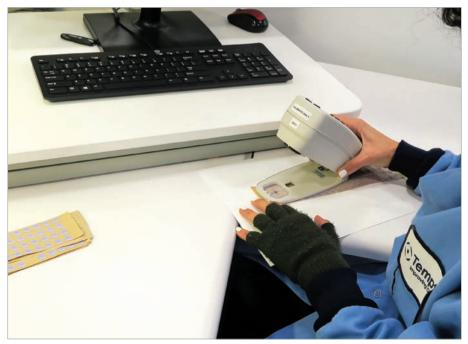
Using X-Rite 500 series spectrodensitometer
