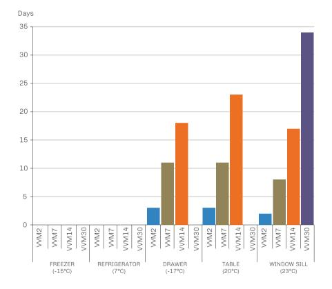
Discard-point in days for four different type VVMs exposed to different conditions
