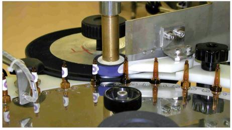
Applying VVMs on the neck of BCG ampoules, Japan BCG
