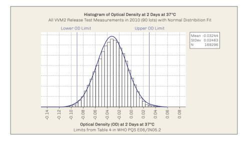
and comparison to specification limits. The tolerance limits include all errors as defined in the specification.
